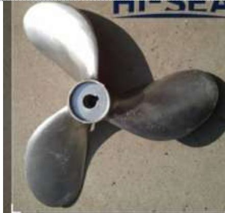
Fig 5 :. Stainless steel based fishing boat propeller
